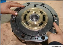
(9) Install casing (1) into assembling jig.
