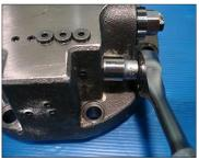
(4) Assemble relief valve (42, 2EA) into rear cover (34).
